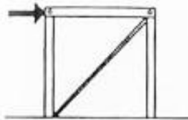
(d) Three basic methods of assuring the lateral stability of simple structural assemblies: diagonal bracing, shear planes, and rigid joints.
